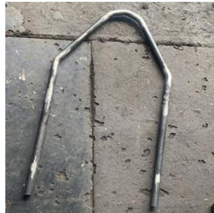
Gambar 3. Roll Bar Mobil Listrik Gambar
